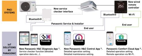
1) A service checker interface is required when this app is used from outdoor location. Wired remote controller (CZ-RTC6BL or CZ-RTC6BLW) is required when this app is used from indoor location. Available from winter 2020, compatible with PZ3 and PZH3 outdoor units. 2) CZ-RTC6BLW required. 3C\_RTC6BLW required. 3C\_RTC6BLW required.
